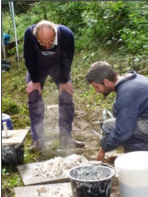
Dirk Bouwens (EARTHA) and Matt Muldoon (right) watching the dry slaking process.
