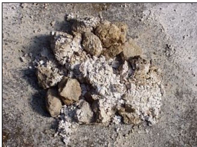
Dry slaking: lumps of quicklime (Calcium Oxide) converting to slaked lime (Calcium Hydroxide) in the presence of water.
